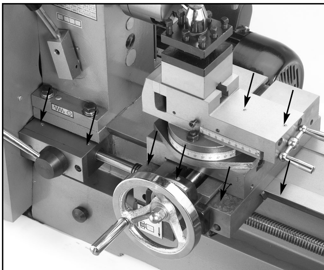
Figure 51. Oil ports indicated by arrows.
